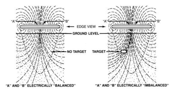
When a target comes within the detection pattern, searchcoils windings become imbalanced at Point A and B, and electromagnetic field lines are redistributed as shown in this drawing.
