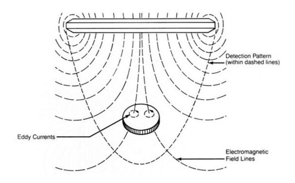
When any metal comes within the detection pattern of a searchcoil, *eddy currents* flow over its surface, resulting in a loss of power in the electromagnetic field, which the detector's circuits can sense.
