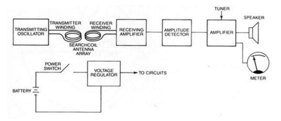
This electronic block diagram of a transmitter-receiver metal detector illustrates the basic
