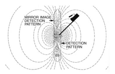
As transmitter current from the antenna generates the electromagnetic field, detection patter (dotted lines) is the area within which Metal detection occurs. Mirror-image pattern atop coil is not used.
