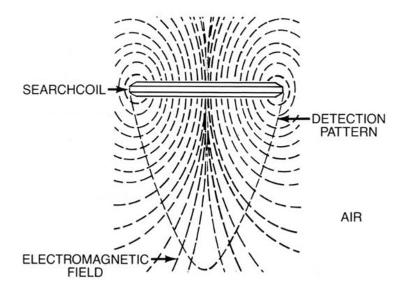
This diagram of "perfect coupling" illustrates the general shape of a detection pattern that occurs when the electromagnetic field from a search coil penetrates earth or any other nearby object.
