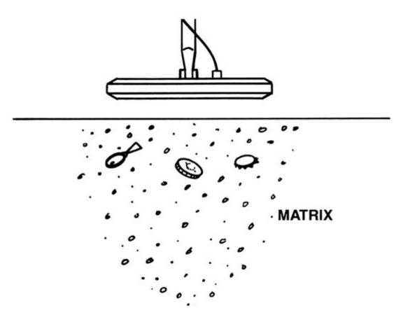
This typical matrix beneath a metal detector's searchcoil illustrates how the electromagnetic field generated by the antenna in that searchcoil illuminates every metal target in the area it reaches.
