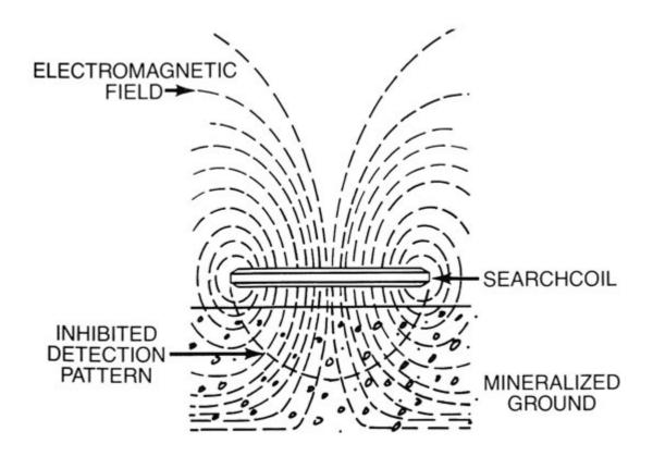
Detection depth capability is inhibited in some elements such as iron mineralization and wetted salt where coupling is inhibited when the electromagnetic field attempts penetration.
