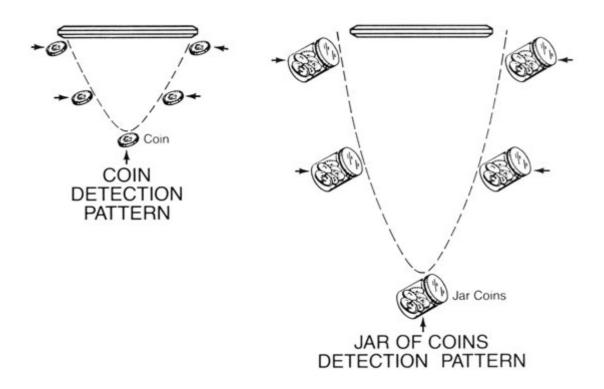
Any detected object has its own pattern, as shown above, with the detection pattern for the jar of coins being wider at the top and extending farther away from the searchcoil's bottom.
